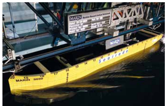
Model test at sea trial condition and a speed of 11 knots
